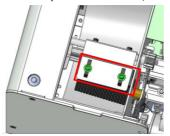
2. Place 5~8 screws into the rail groove close to the holding plate rear end and loosen 2 screws on the side of the brush bracket. Swing the brush and adjust the height until the brush just touch the screw heads slightly, and tighten the screws after adjustment.
